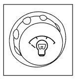
Press this knob located next to the exterior lamps knob to extend it, and then turn it to adjust the instrument panel brightness.
